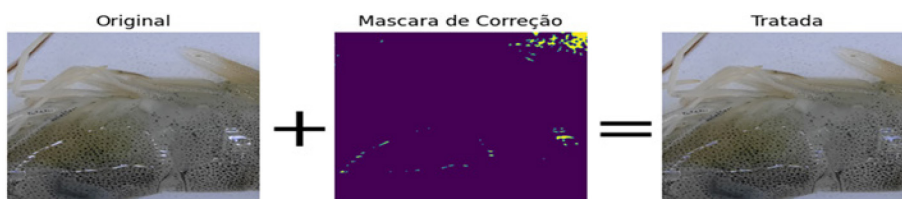
Figure 7. Images showing the focus of item I in figure 5, through thresholding to reduce light noise, in which each line has a process (from left to right), verifying that the luminosity no longer appears after applying the mask. Source: Authors, 2025.
