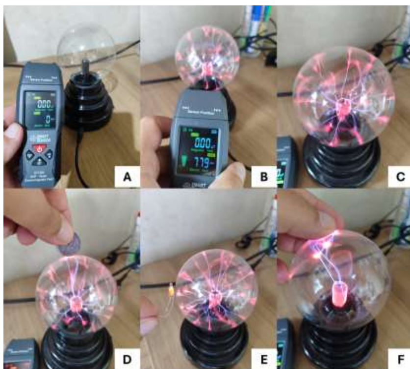
Figure 3. Simple experiments with a plasma ball: analysis of electric and electromagnetic fields using a detector, a metallic coin, a neon lamp, and human skin contact. Source: Author, 2025.
