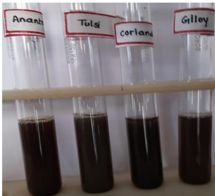
Figure 2. Synthesized Silver nanoparticles. Source: Authors, 2024.
