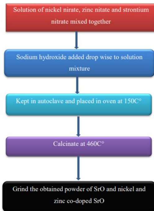
Figure 1. Schematic synthesis of Strontium oxide nanoparticles was conducted using a hydrothermal method.
