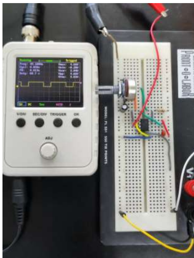
Figure 6. On the right, the circuit assembled on the breadboard, on the left we can see the oscilloscope reading the output signal. Source: Author, 2023.
