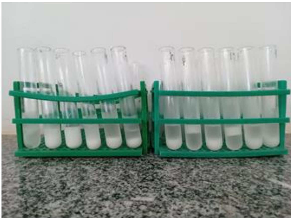
Figure 3. Solubility test in different solvents on Manilkara zapota latex. Note: From left to right, water, ethanol, methanol, acetone, hexane, ethyl ether, petroleum ether, chloroform, ethyl acetate, dichloromethane, toluene and xylene. Source: Authors, 2022.
