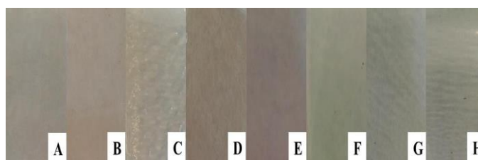
Figure 1. Arrowroot starch films incorporating floral extract of Tabebuia impetiginosa and copper solution. A: B: C: D: E: F: G: H: Source: Authors, 2021.
